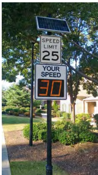
3) Digital speed radar sign
