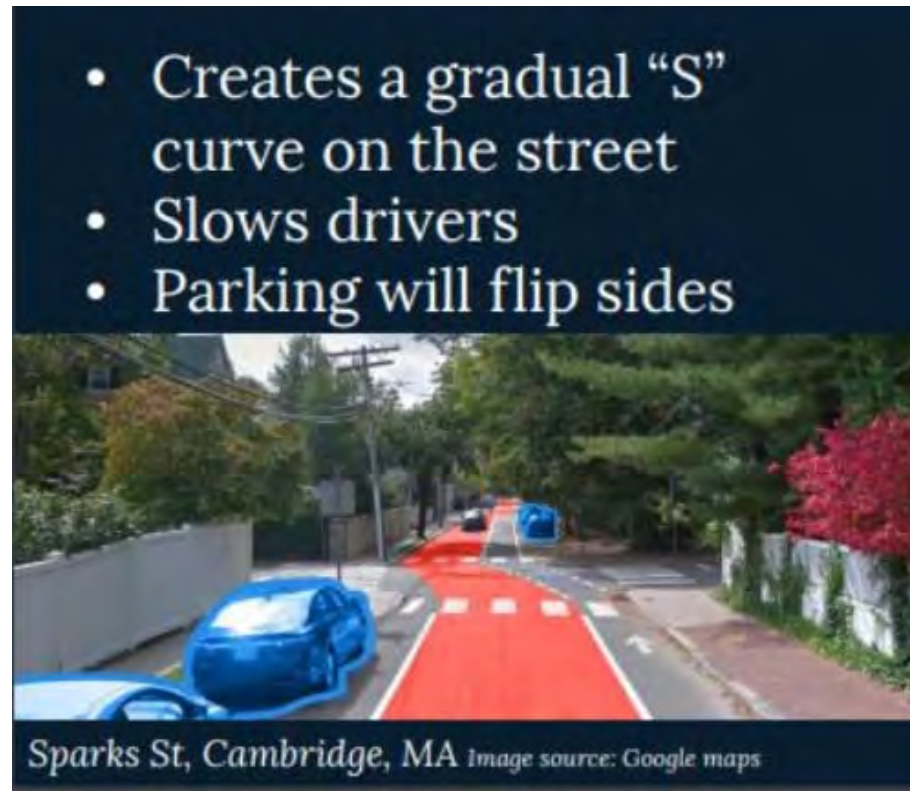
1) Chicane using on-street parking
