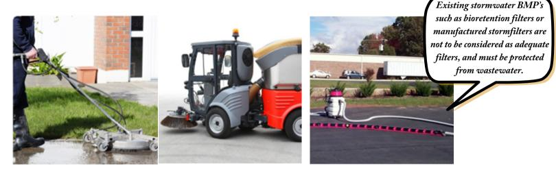
Other options include rotary cleaners that supply high pressure water and collect dirty wash water in an attached storage tank, vacuum booms or berms that seal to the ground and suck washwater through a hose to also collect in a storage tank, and ride-on surface cleaning vehicles that collect and recycle washwater
