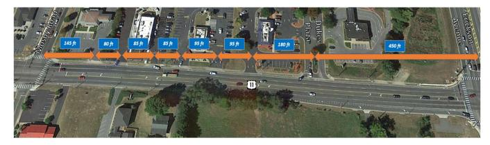
Figure 16: Existing Commercial Access Spacing
