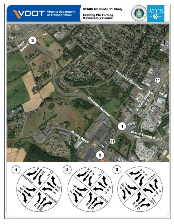
Figure 2: Study Intersections Existing Turning Movement Counts
