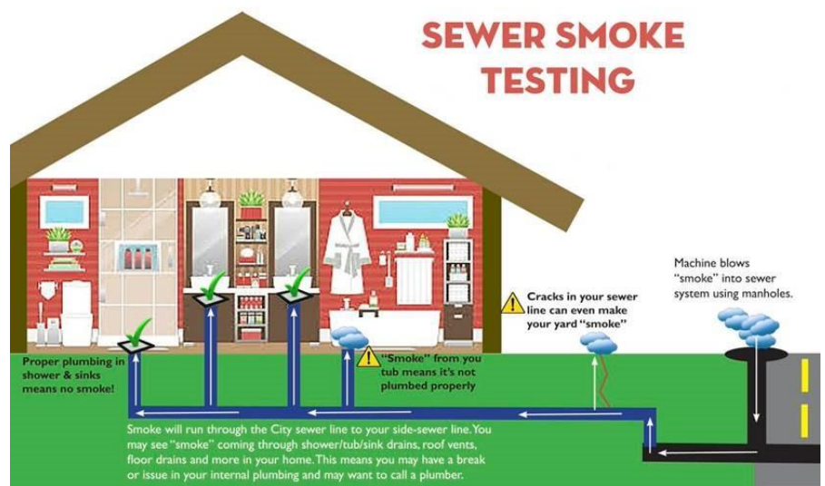
(Above) This graphic shows how the annual testing works, and where residents may notice some smoke.
