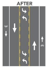
of lanes. Most commonly, a road with two lanes in each direction is reconfigured to have one lane in each direction, a center turn lane and bicycle lanes in each direction, along with necessitated storage lanes or additional turn lanes where needed (see above image for example).
