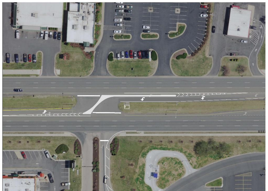
Crews will construct a restricted crossing U-turn at a median crossover on East Market Street starting Monday. (Above) This rendering shows how the new crossing will function.
