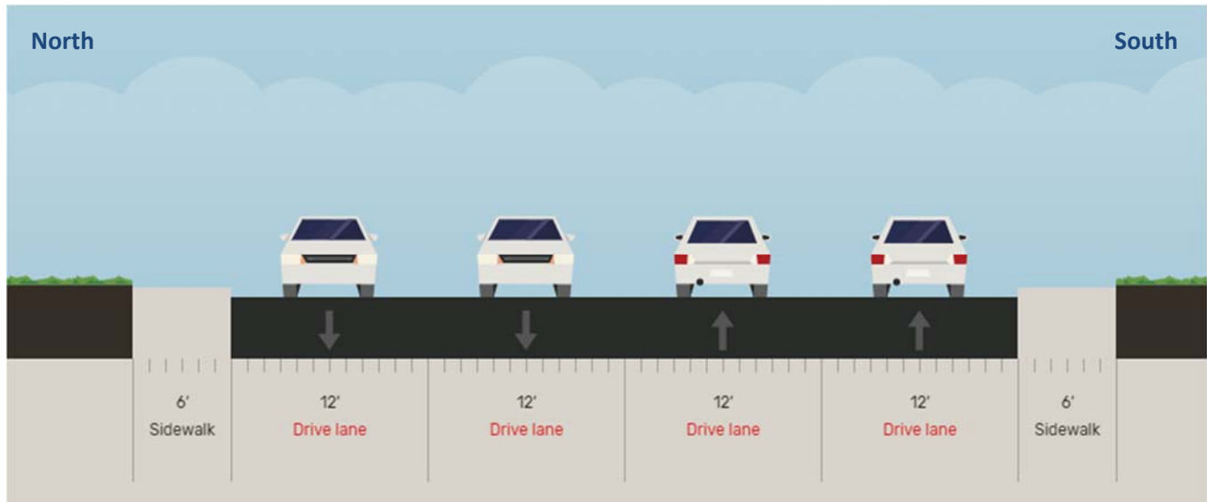
Figure 5: E Market Street Existing Cross Section
