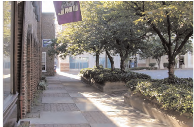
Raised concrete planter walls isolate shop fronts from street and Court Square context. The streetscape plan calls for replacement of the raised planters with flush street trees and integration of the sidewalk with a grand Courthouse Square urban plaza.
