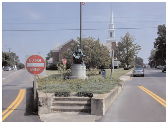
Investigate relocation of “Do Not Enter” sign to north corner of monument or via street markings.
