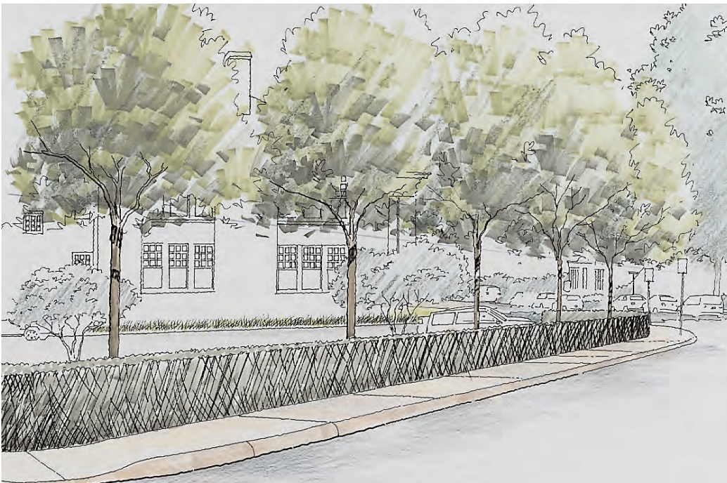
View of Harrisonburg City Hall from Main Street. Perspective sketch shows addition of shade trees and hedge to screen parking. Landscape buffering of parking should be a required standard for all proposed downtown parking.
